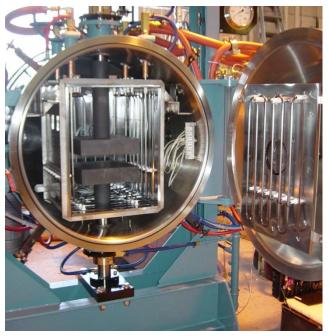
processing environments are available including high/low vacuum and partial and/or positive pressures of Ar, He, and N2 gases, or H2 process gas with our G-10503A gas system.
