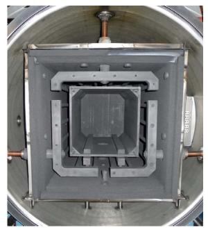
cost designs using graphite 'slat' elements bolted to the phase bar which can loosen over time causing micro-shorts and poor temperature uniformity.
