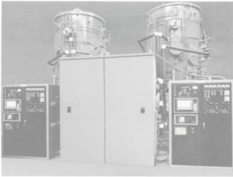
Fig. 5. Tandem 24" Diameter by 36" High CVD Furnaces With Common Power Supply
