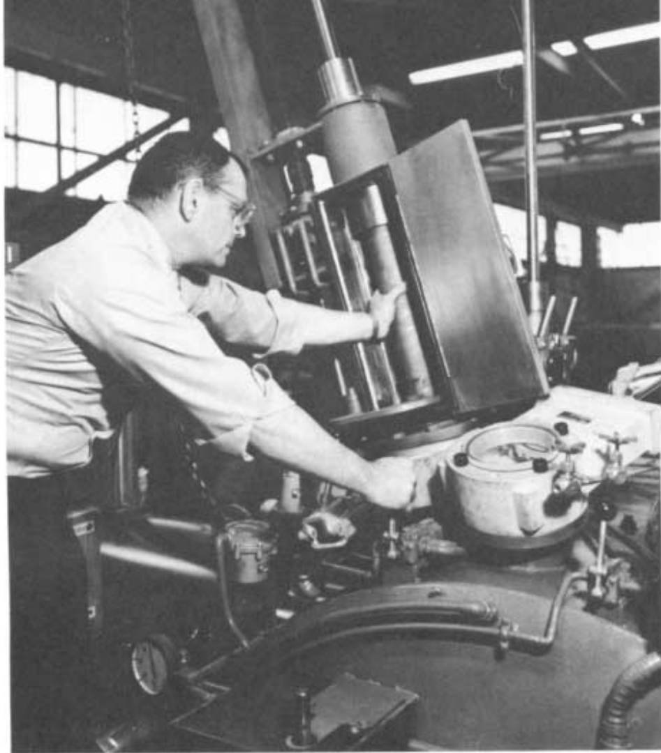
Fig. 2—Operator loads a billet into the billet charger. Note valved operator's view port, immersion thermocouple, and miscellaneous controls.
