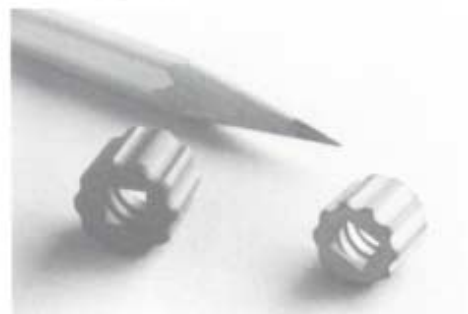
FIG. 2 Stainless steel threaded insert in green and sintered condition.
