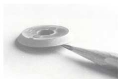
FIG. 3 Tungsten carbide splitter knife. Moulding and sintering reduces secondary operations.
