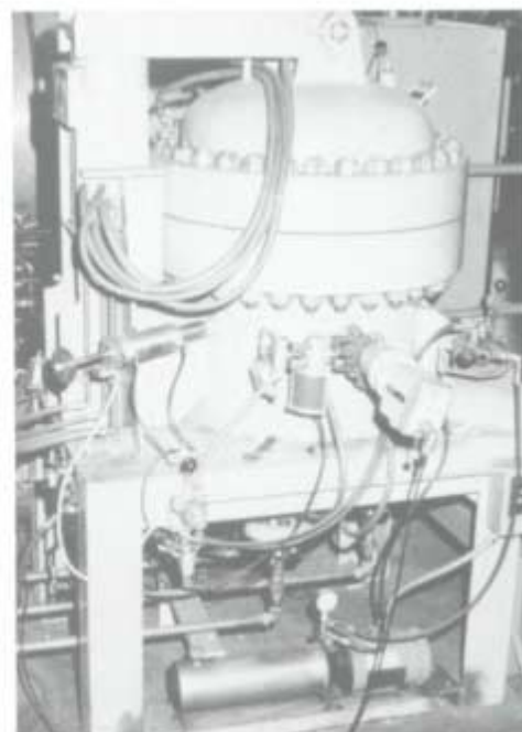
FIG 8 Side view - 2200C, 100 bar, 15 liter carbon-free furnace
