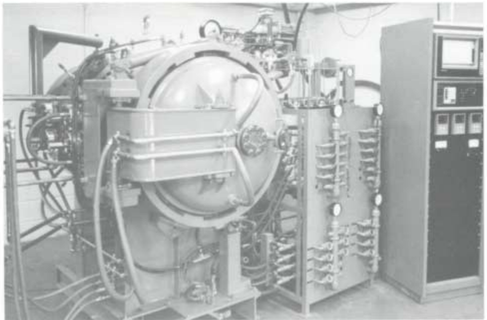
FIG 1 Early design SINTERBAR™ combination delube, sinter, pressure densification furnace
