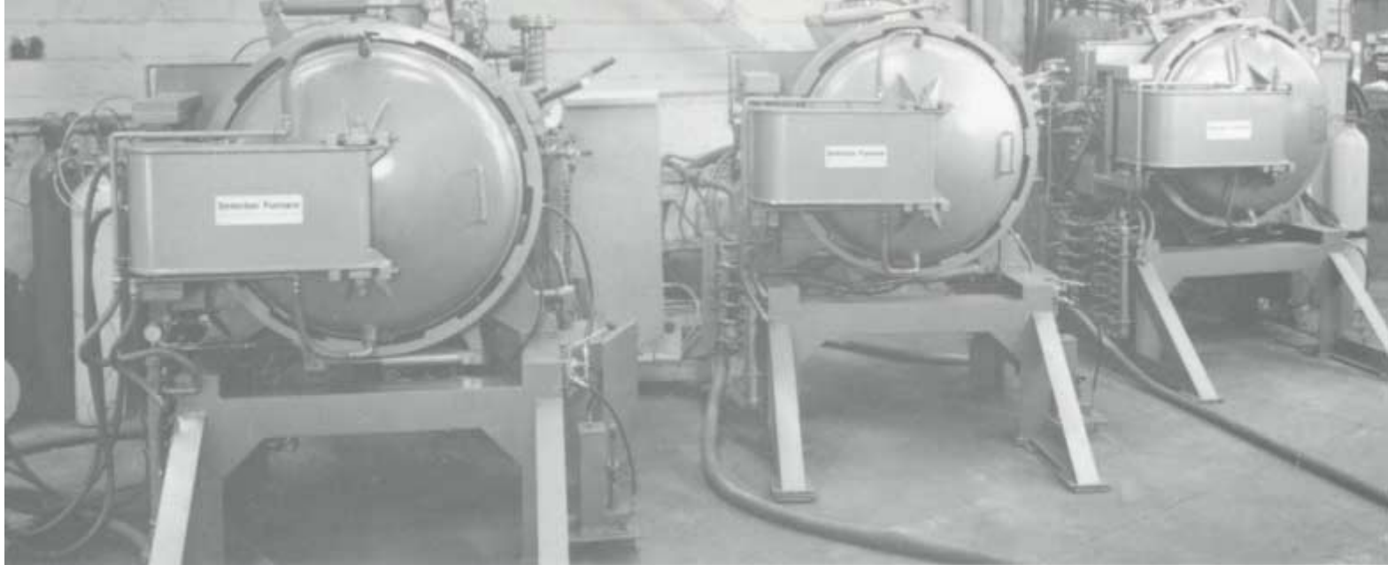
FIG 6 Three pilot plant pressure furnaces for binder removal, reaction bonding, sintering silicon nitride
