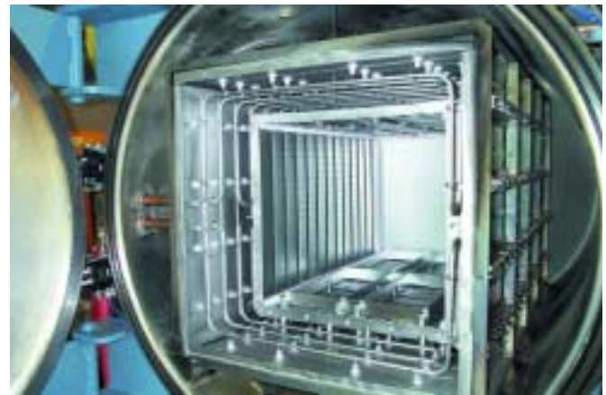
Metal hot zone in MIM sintering furnace
