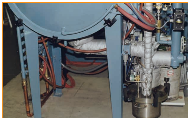
Figure 14: Centorr/Vacuum Industries' positive pressure hydrogen gas debinding system.
