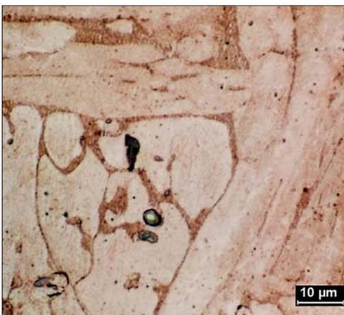
Fig. 9 Microstructure of part with 97% theoretical density
