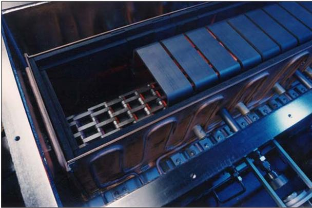
Fig. 11 Graphite hot zone and SiC belt in ceramic belt furnace
