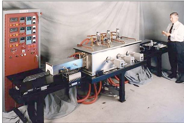
Fig. 6 Centorr Vacuum Industries belt furnace for the processing of advanced metals and ceramics
