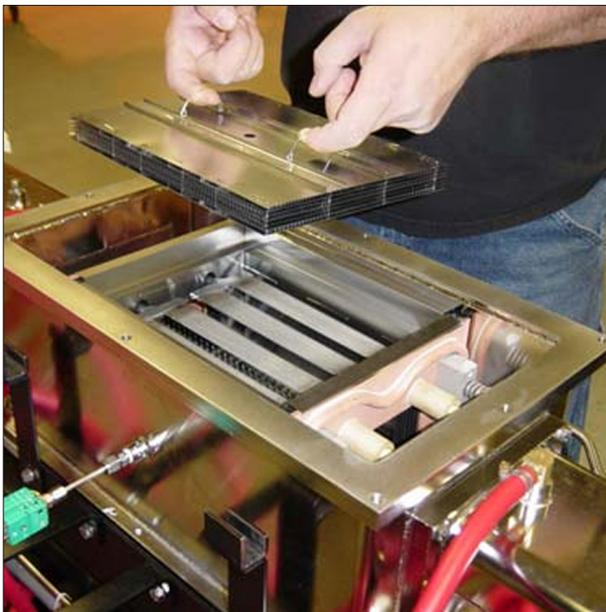
Fig. 3 Refractory metal belt furnace hot zones
