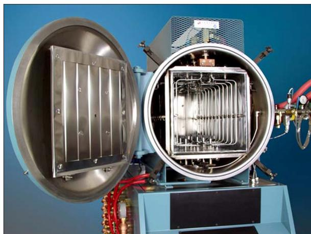
Fig. 1 Conventional vacuum furnace hot zone
