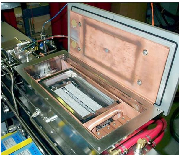
Fig. 4 Refractory metal belt furnace hot zones
