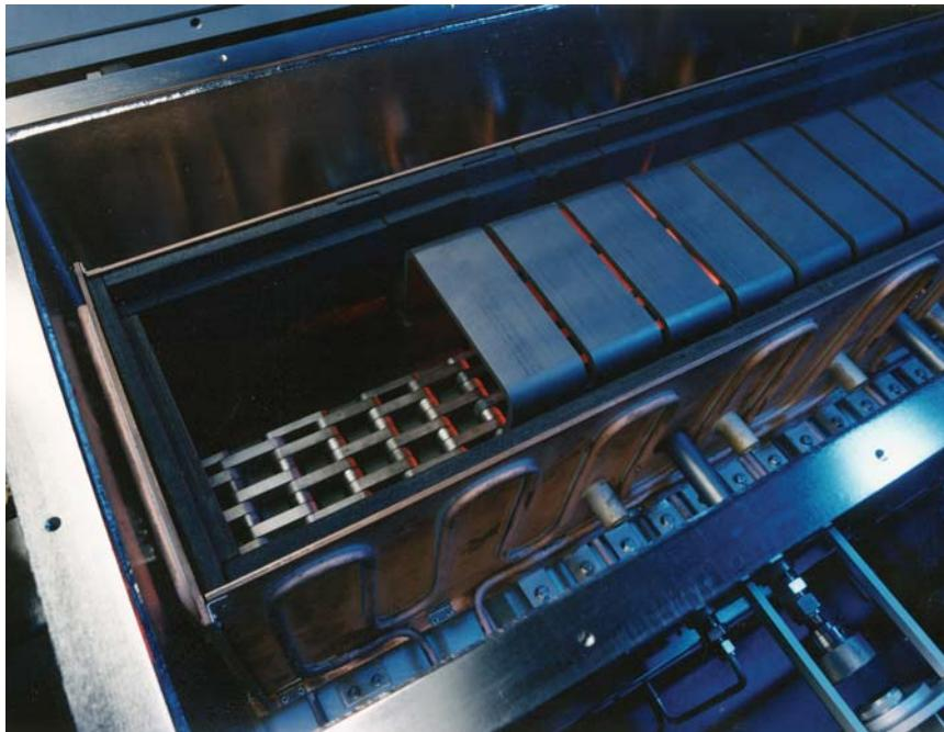
**Fig. 7. Graphite hot zone and SiC belt in ceramic belt furnace**
