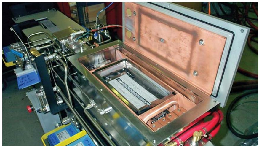
**Fig. 3. Refractory-metal belt-furnace hot zones**
