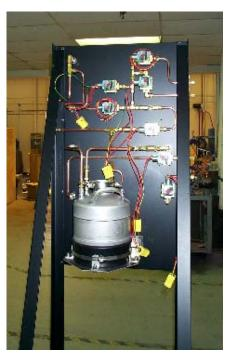
Design should include copper piping with brass fittings for inert gas and Hydrogen for dew point monitoring above -20°C. If dissociated ammonia is the process gas, system should use all SS piping. If dewpoints less than -20°C are desired, all SS piping (for either inert or H2) should be used with Swagelock fittings for all connections. VRC fittings or orbital welding available upon request at extra cost.
