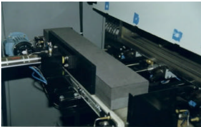
Graphite workbox being transferred to entrance load lock.
