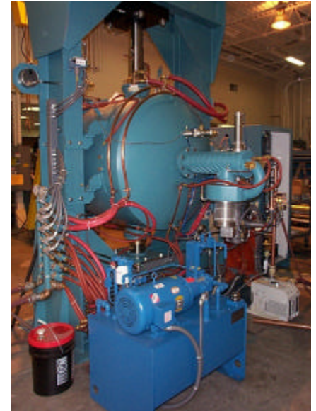
Hydraulic power supply, fan cooling system and diffusion pumping system.
