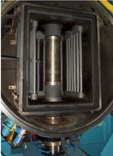
Series 3600 Model 191919-2300-300T with steel dogbone for testing ram force.
