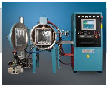
comprises of three standard hot zone sizes in four different temperature ranges (1000°C, 1315°C, 1650°C, and 2000°C), with a long list of optional equipment that makes this one of the most versatile custom-designed furnaces available today. The furnace chamber is mounted on legs for a compact and highly efficient design and is a "front-loading" orientation which offers better ergonomics and temperature uniformity compared with vertical top/bottom loaders or round hot zones.
