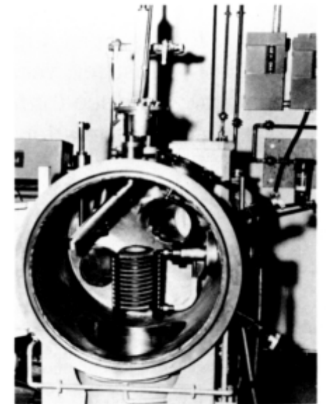
Fig. 3. The melt chamber for a 17-lb capacity VIM furnace.
