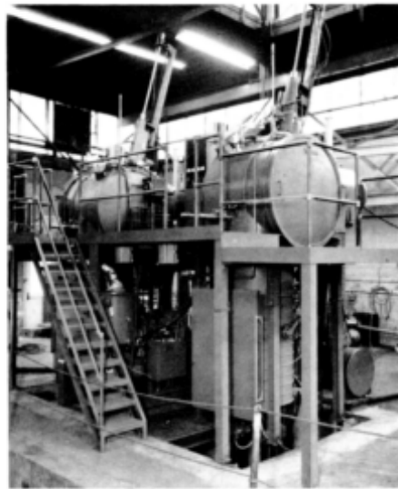
Fig. 1. Twin 50-lb capacity VIM furnaces form part of semicontinuous system for production melting.
