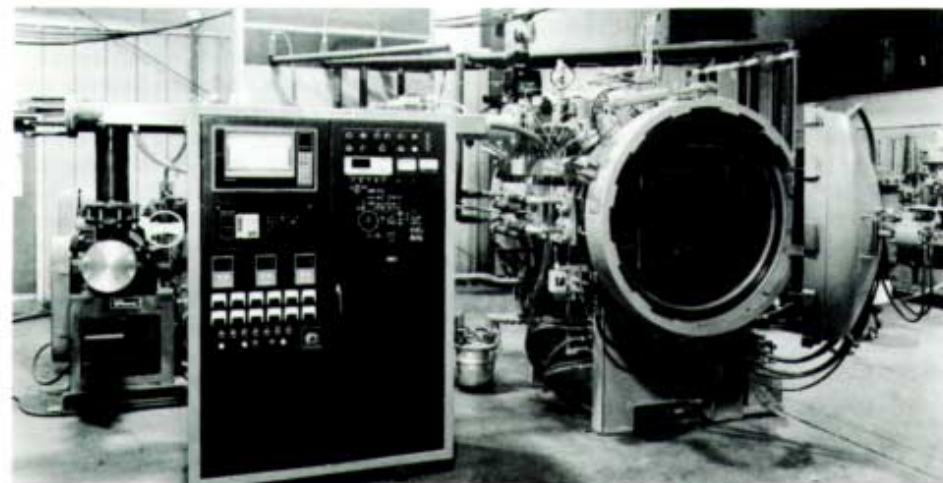
FIG. 2 'Sinterbar' 300 furnace. Temperatures to 1600C with graphite resistive heating and pressure to 400 psig (27.5 bar).
