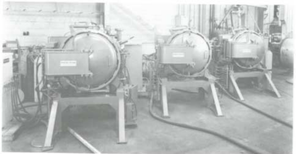
FIG. 5 Three 'Sinterbar' furnaces for binder removal, reaction bonding, and high temperature, high pressure sintering of silicon nitride parts.
