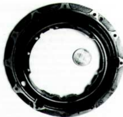
FIG. 8 Stainless steel gyroscope support ring sintering density 7.4 gm/cc.
