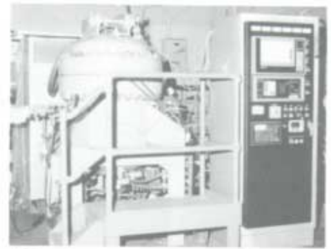
FIG. 4 'Sinterbar' vertical loading furnace with temperature capabilities of 2200C and pressures to 1500 psig (100 bar).
