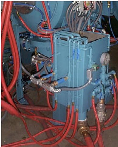
Photograph of open drain water system with drain bosh.
