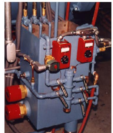
Photograph of open drain system with hot water option.
