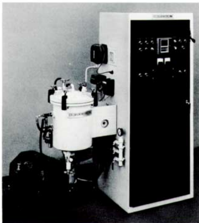
Sintervac® laboratory and quality control furnace with modular chamber/control cabinet and vacuum pump.
